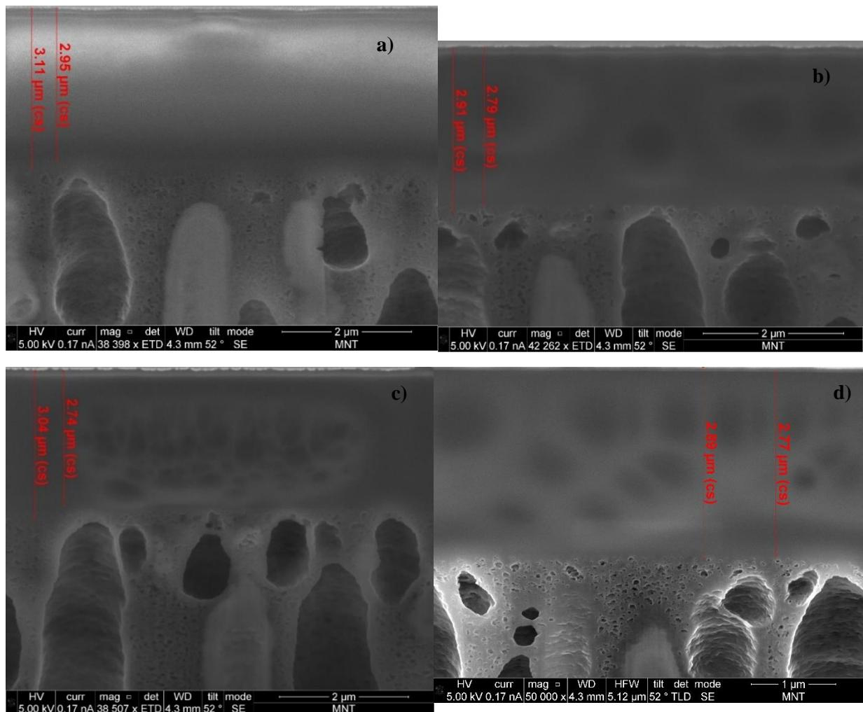
**Figure A.6.** FIB-SEM images of PDMS-PVA-TiO<sub>2</sub> membrane: a) fresh, b) exposed at 40 °C, c) exposed at 60 °C, and d) used in dehydration of ChCl-urea.
