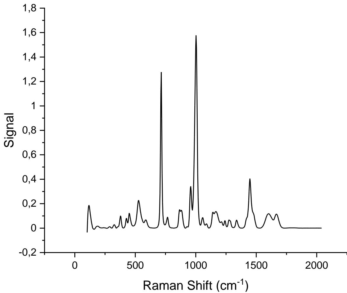
**Figure A.7.** Raman spectrum of 90% ChCl-urea feed solution.
