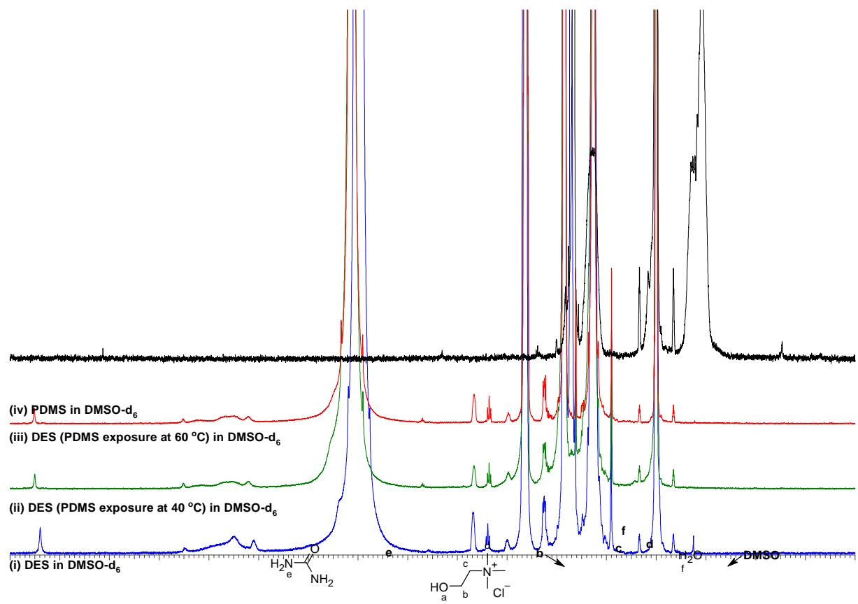
**Figure A.1.** <sup>1</sup>H NMR spectra of fresh DES (i), exposed DES samples (ii and iii), and PDMS (iv) in DMSO-d<sub>6</sub>.
