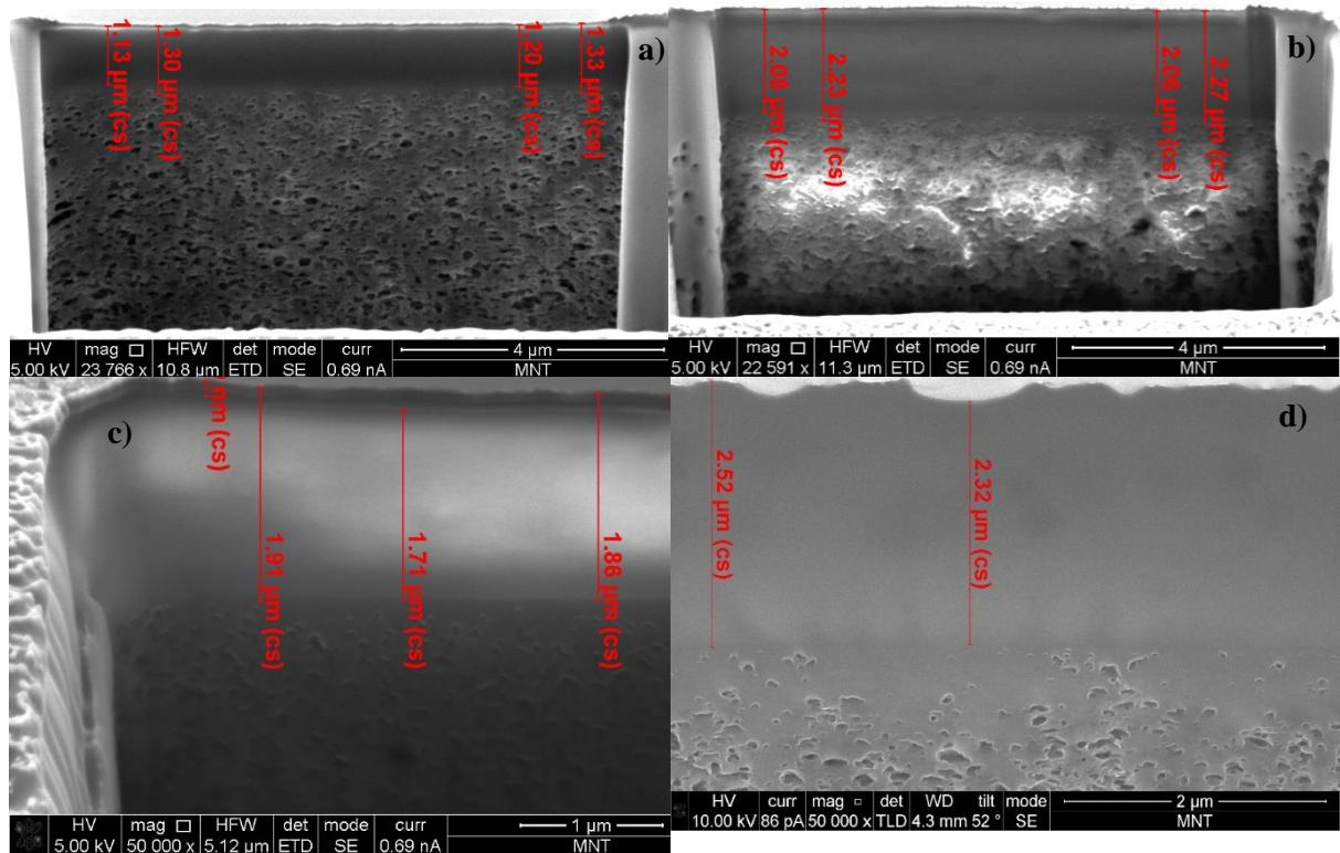
**Figure A.4.** FIB-SEM images of PERVAP 4155-80 membrane: a) fresh, b) exposed at 40 °C, c) exposed at 60 °C, and d) used in dehydration of ChCl-urea.
