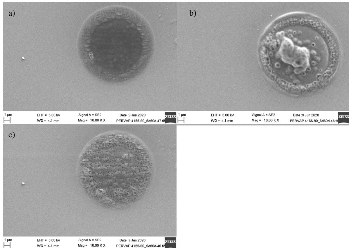
**Figure A.3.** FESEM images of a location with ChCl-urea inside the membrane structure and bubbling with 10,000 x magnification. The images were taken in series; first a) and as last c). The bubbling of ChCl-urea may have been caused by the higher intensity of the several electron beam scans as the scanning focus is on a relatively small surface area when high magnifications are used; and in addition, by vacuum in the sample compartment.
