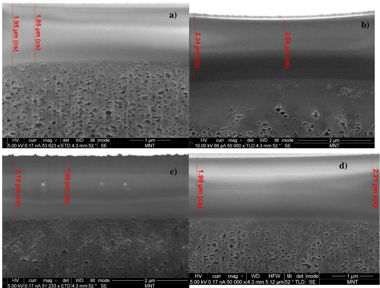
**Figure A.5.** FIB-SEM images of PDMS membrane: a) fresh, b) exposed at 40 °C, c) exposed at 60 °C, and d) used in dehydration of ChCl-urea.
