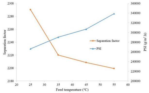
Fig. 7. The effect of feed temperature on the separation factor and PSI (feed concentration: 34.41 ppm, membrane thickness: 58.41  $\mu\text{m}$ )
