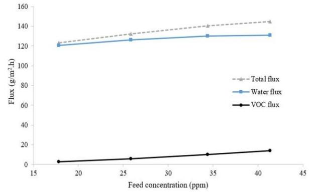
Fig. 3. The effect of feed concentration on 2-ethyltoluene, water, and total fluxes (membrane thickness: 52.03 μm, feed temperature: 25 °C)
