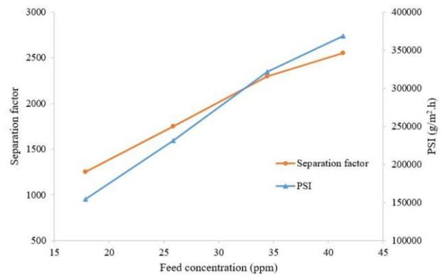
Fig. 4. The effect of feed concentration on the separation factor and PSI (membrane thickness: 52.03 μm, feed temperature: 25 °C)
