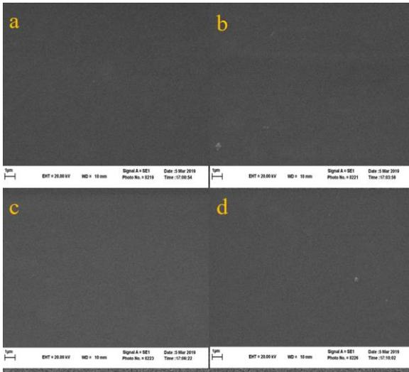
Fig. 1. SEM surface images of the membranes with different thicknesses: a) 46.09 μm, b) 52.03 μm, c) 58.41 μm, and d) 63.97 μm
