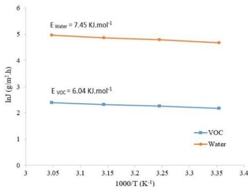
Fig. 6. Arrhenius plots of components flux
