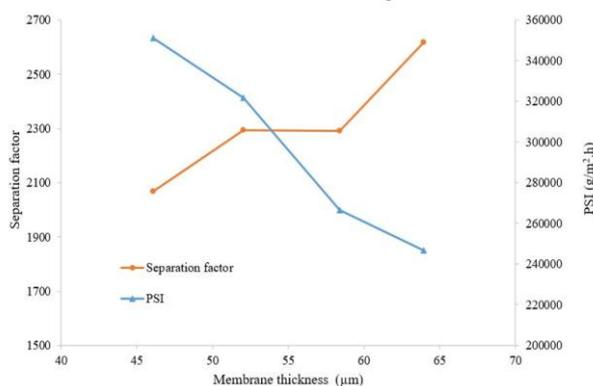
Fig. 9. The effect of membrane thickness on the separation factor and PSI (feed concentration: 34.41 ppm, feed temperature: 25 °C)
