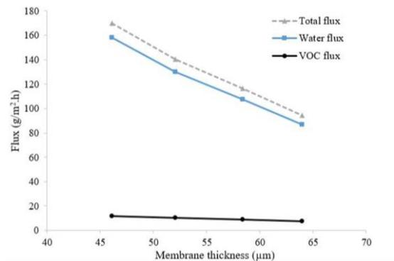
Fig. 8. The effect of membrane thickness on 2-ethyltoluene, water, and total fluxes (feed concentration: 34.41 ppm, feed temperature: 25 °C)
