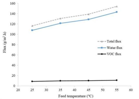
Fig. 5. The effect of feed temperature on 2-ethyltoluene, water, and total fluxes (feed concentration: 34.41 ppm, membrane thickness: 58.41  $\mu\text{m}$ )
