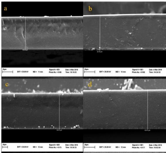
Fig. 2. SEM cross-sectional images of the membranes with different thicknesses: a) 46.09 μm, b) 52.03 μm, c) 58.41 μm, and d) 63.97 μm
