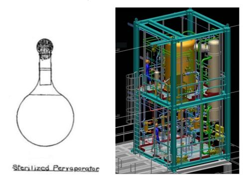
Fig. 1. The evolution of pervaporation; from a collodion bag (adapted with permission from [1], copyright 2017 American Chemical Society) to a skid-mounted plant [2].
