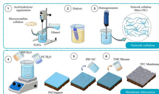
Fig. 1. Schematic illustration of membrane fabrication steps.
