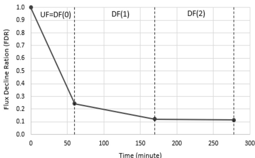
Fig. 9. Flux decline ratio at different stages of DF experiment for 15kDa membrane.
