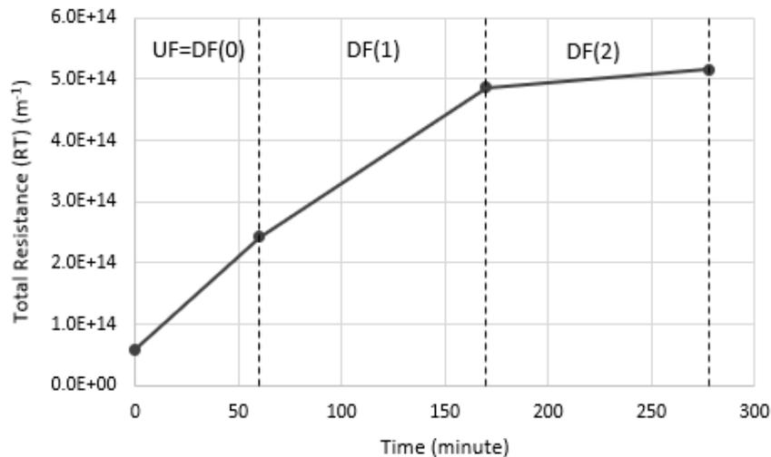
Fig. 8. Total resistance values at different stage of DF experiment for 15kDa membrane.
