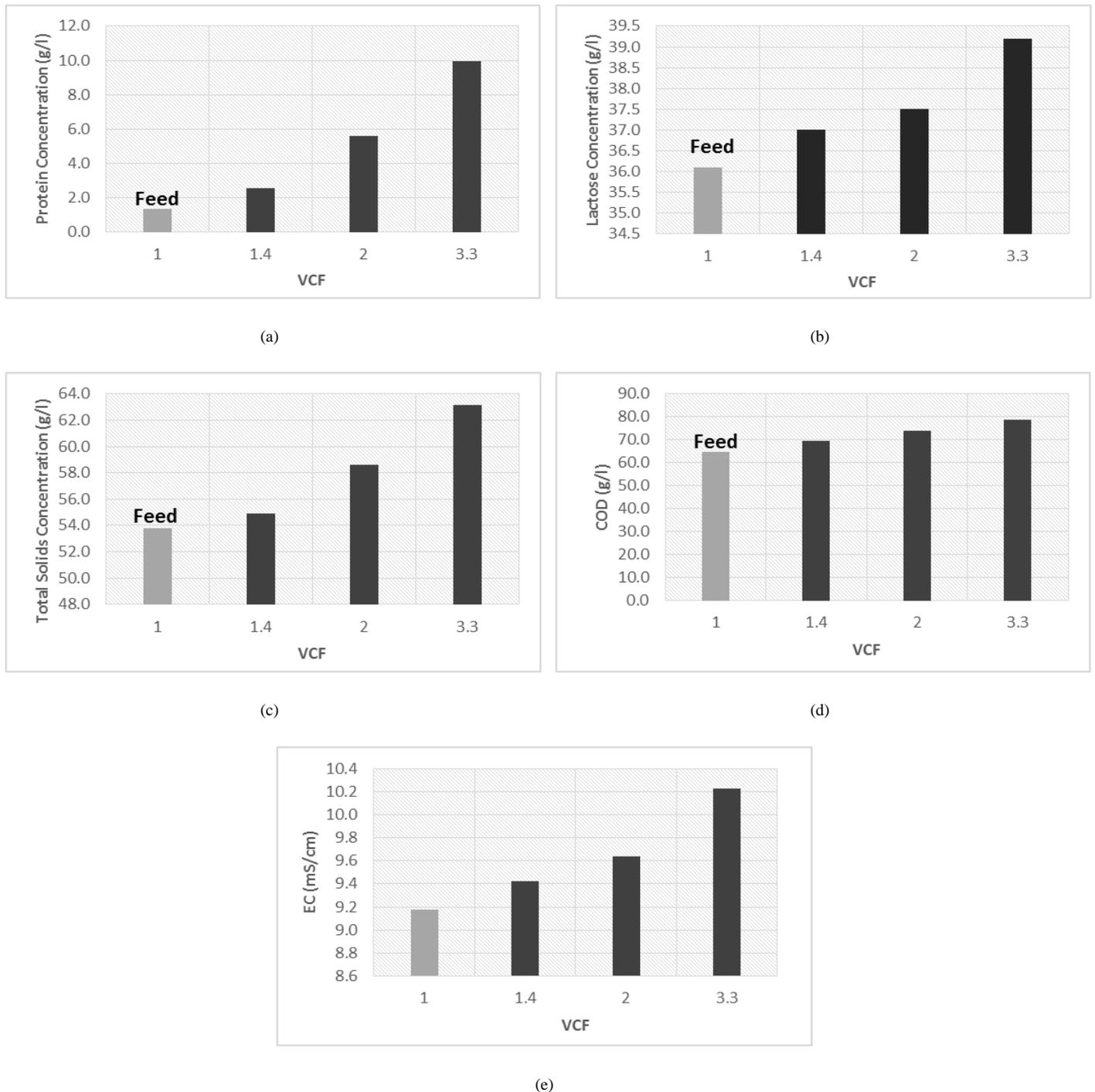
Fig. 3. Concentration in concentrate stream of (a) Protein (b) Lactose (c) Total solids (d) COD (e) Electrical conductivity with different VCF values for 15kDa MWCO.
