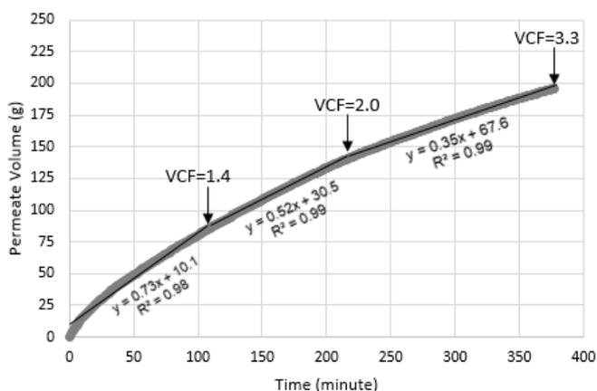
Fig. 2. Permeate volume curve for different VCF values of 15kDa membrane.
