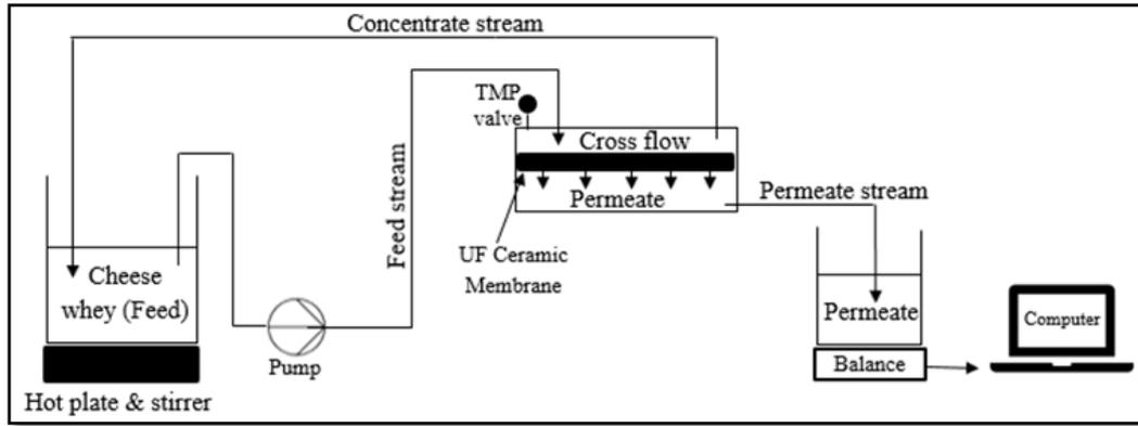
Fig. 1. A general scheme of the cross flow filtration system.
