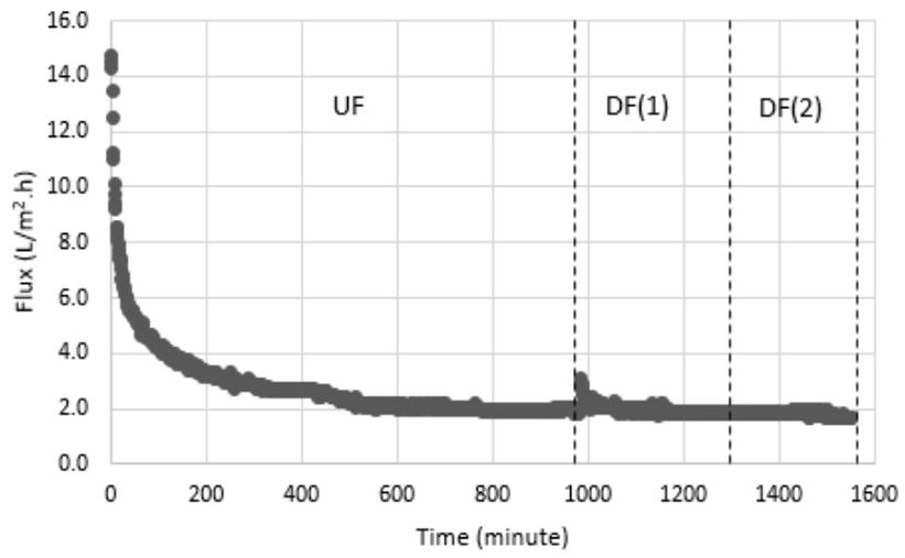
Fig. 4. Flux curve of DF experiment with two DF cycles and 3.3VCF of UF.
