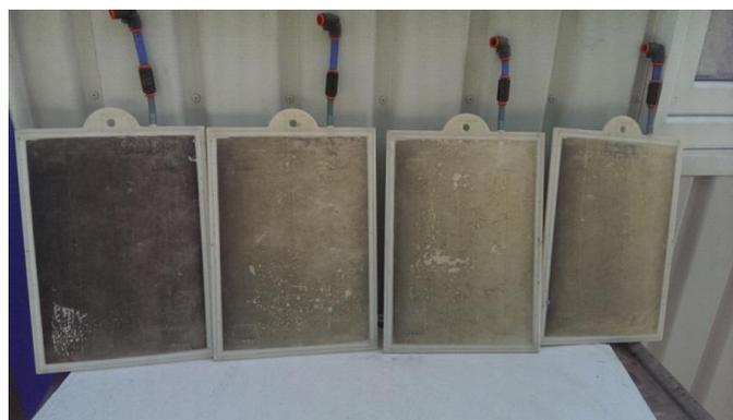
**Fig. 4.** Fouling on MBR membranes after 29 days of operation in tap water in the absence of antiscalant.
