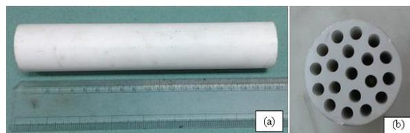
Fig.8. Support tube images (a) horizontal and (b) cross sectional view.
