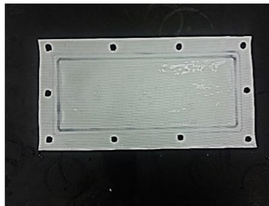
Fig. 5. Gelation layer on membrane surface at inlet velocity of (a) 0.064 m/s and (b) 0.297 m/s.
