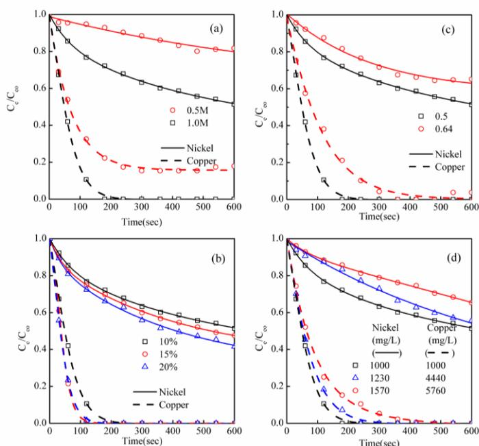
Fig. 3. Effect of parametric variables on the co-extraction of copper and nickel from ammoniacal media in ELMs. (a) Effect of internal phase acid concentration ( $C_{i0}$ ), (b) Effect of carrier concentration ( $C_c$ ), (c) Effect of internal phase volume fraction ( $\phi$ ), (d) Effect of initial copper and nickel concentration in feed ( $C_{\infty}$ ) (Conditions as in Table 2).
