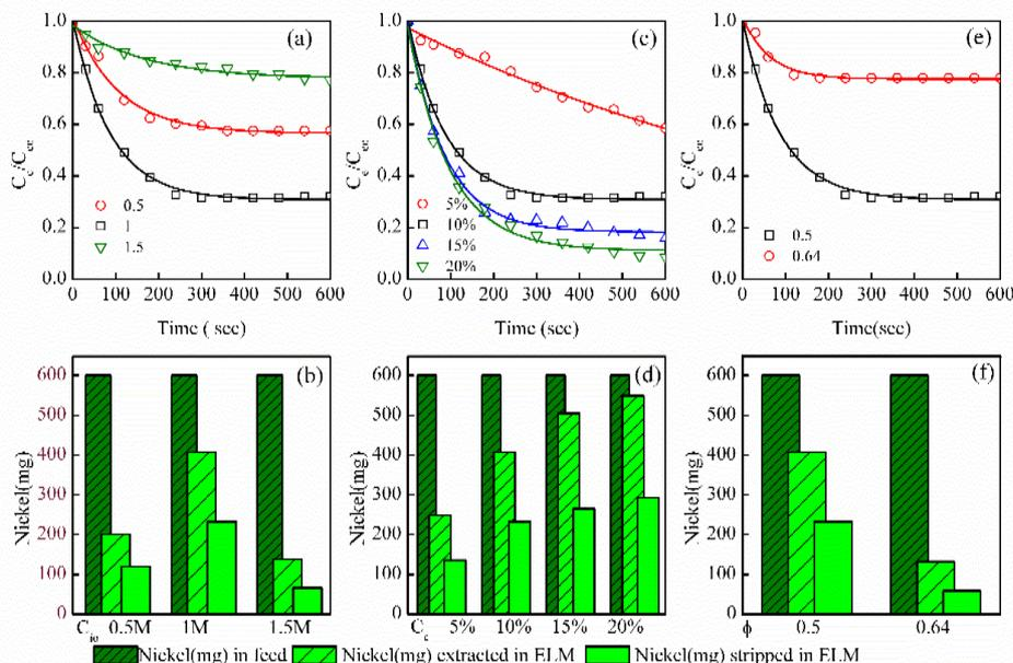
Fig. 2. Effect of emulsion parameters on the extraction and stripping patterns of nickel from ammoniacal media into ELMs. (a), (b) Effect of internal phase acid concentration ( $C_{io}$ ), (c), (d) Effect of carrier concentration ( $C_c$ ), (e), (f) Effect of internal phase volume fraction ( $\phi$ ) (Conditions as in Table 1).
