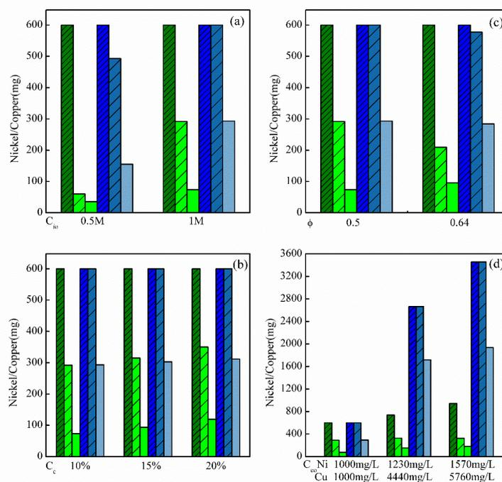
Fig. 4. Copper-nickel, extraction-stripping patterns in ELMs, (a) Effect of internal phase acid concentration ( $C_{10}$ ), (b) Effect of carrier concentration ( $C_c$ ), (c) Effect of internal phase volume fraction ( $\phi$ ), (d) Effect of initial copper and nickel concentration in feed ( $C_{00}$ ).
