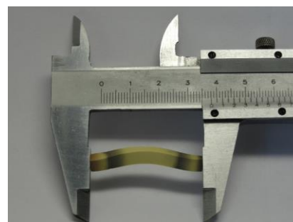
Fig. 3. Photography of \text{In}_2\text{O}_3\text{-48 wt.% Bi}_2\text{O}_3 LGBS after deformation at 840 °C.
