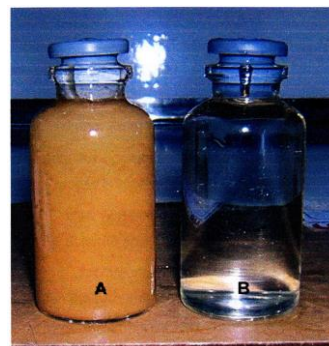
Fig. 8. Visual sample observation of (A) mixed liquor and (B) permeate from MBR.
