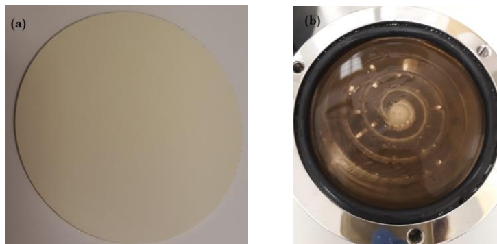
Fig. 12. The new Ceram 0.45 μm ceramic membrane (a) and the filtration cake formed on its surface during the treatment of the digestate liquid fraction (b).
