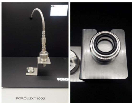
Fig. 3. The POROLUX™1000 porometer with a sample holder used in this study
