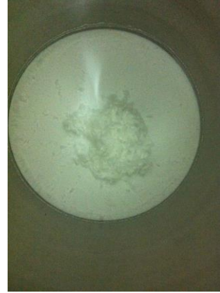
Fig. 4. Picture of the caffeine crystals grouped on the membrane surface.
