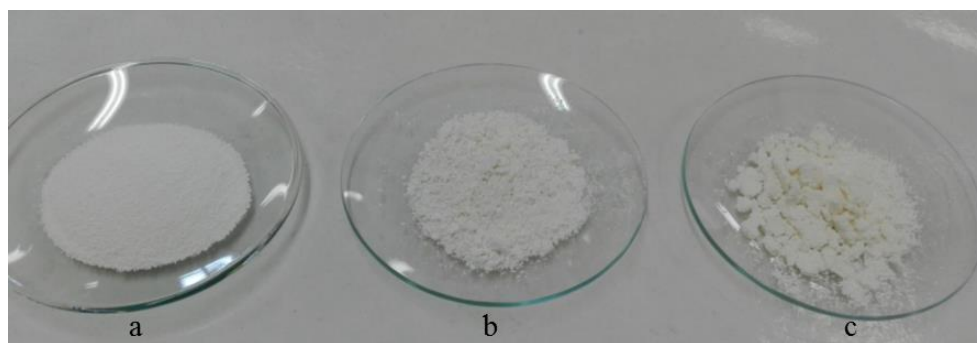
Fig. 3. Effect of reagent concentration on polymer powder appearance: a) Pure PES, b) DG= 22.4%, and c) DG= 20.2%. It is imperative to note the aggregations of powder that start forming from b).
