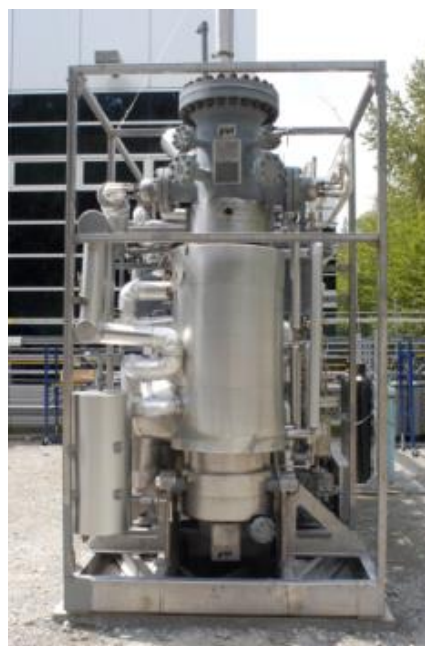
Fig. 8. Internally circulating FBMR for hydrogen production.
